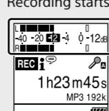
During recording, the peak level meters appear to help you adjust the recording level (A).
